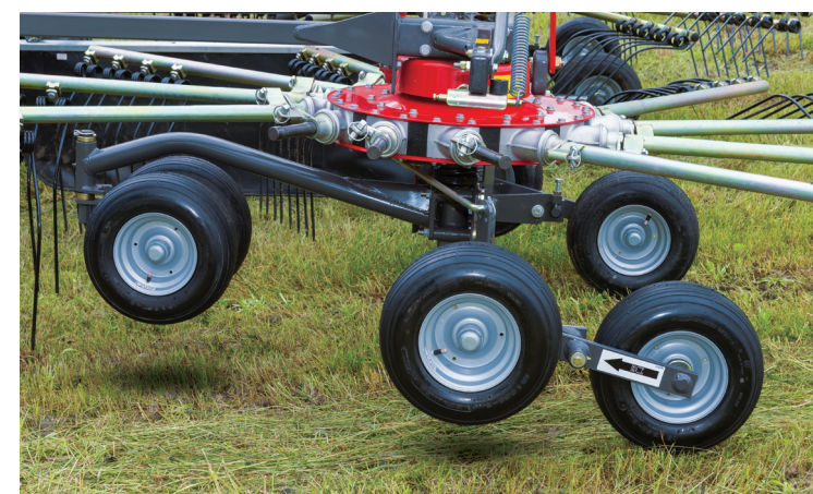
Patented, fully cardanic rotor suspension
