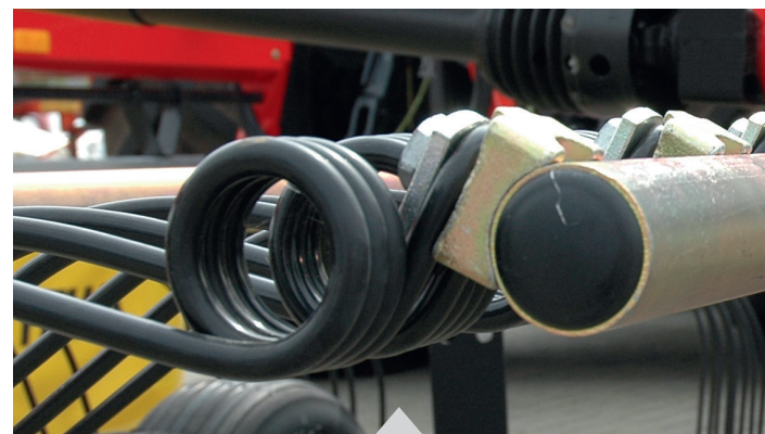
Absolutely smooth front side of the tine arm
